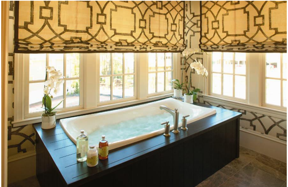
FIGURE 15.10 These windows are designed to provide views; however, window treatments are needed for control of solar gain and privacy.
