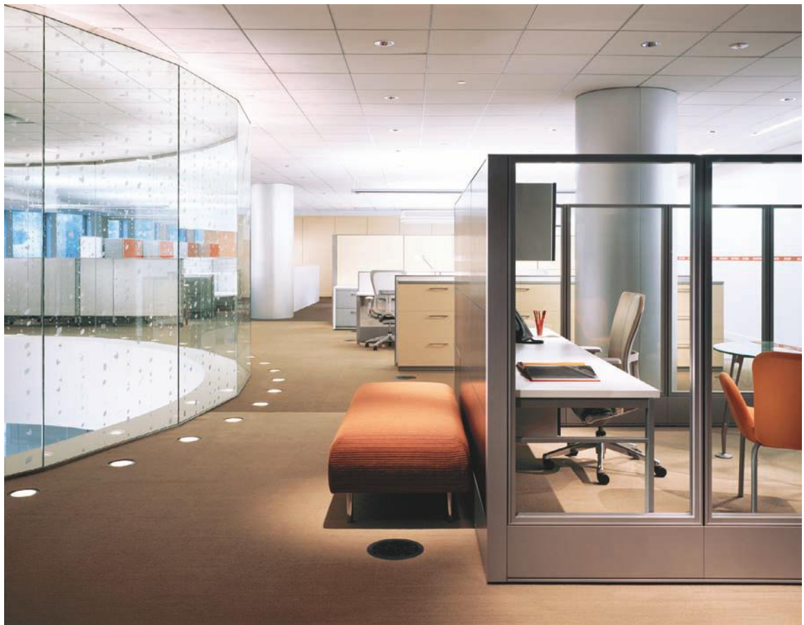
FIGURE 16.28 High, glazed panels are used for this office to provide privacy and collaborative spaces without building full-height walls.
