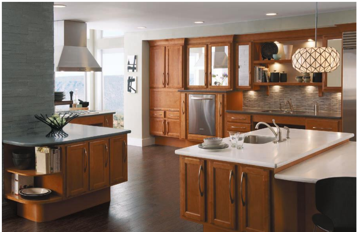
FIGURE 8.42 One of the main features in this accessible kitchen is cabinets raised off the floor, with a deep toe-kick, to provide easy wheelchair access. Other features include a raised dishwasher and pull-out cabinets.
