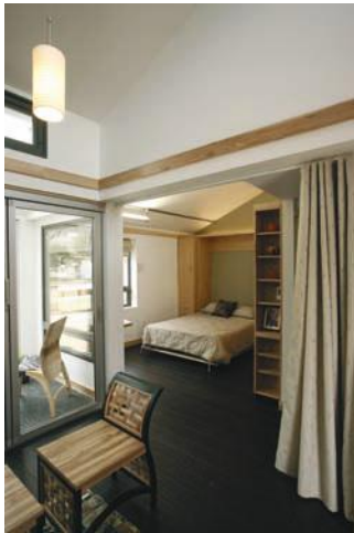
FIGURE 8.24 This fold-up bed provides additional floor space in a small house when it is put away.
