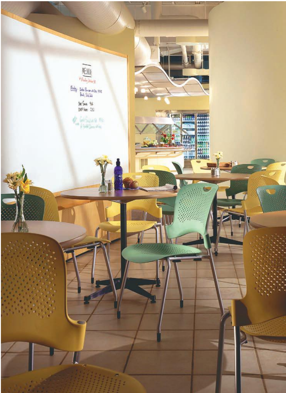
FIGURE 14.15 Ceramic tiles can be used for durable and scrubbable floor surfaces, as seen in this cafeteria.
