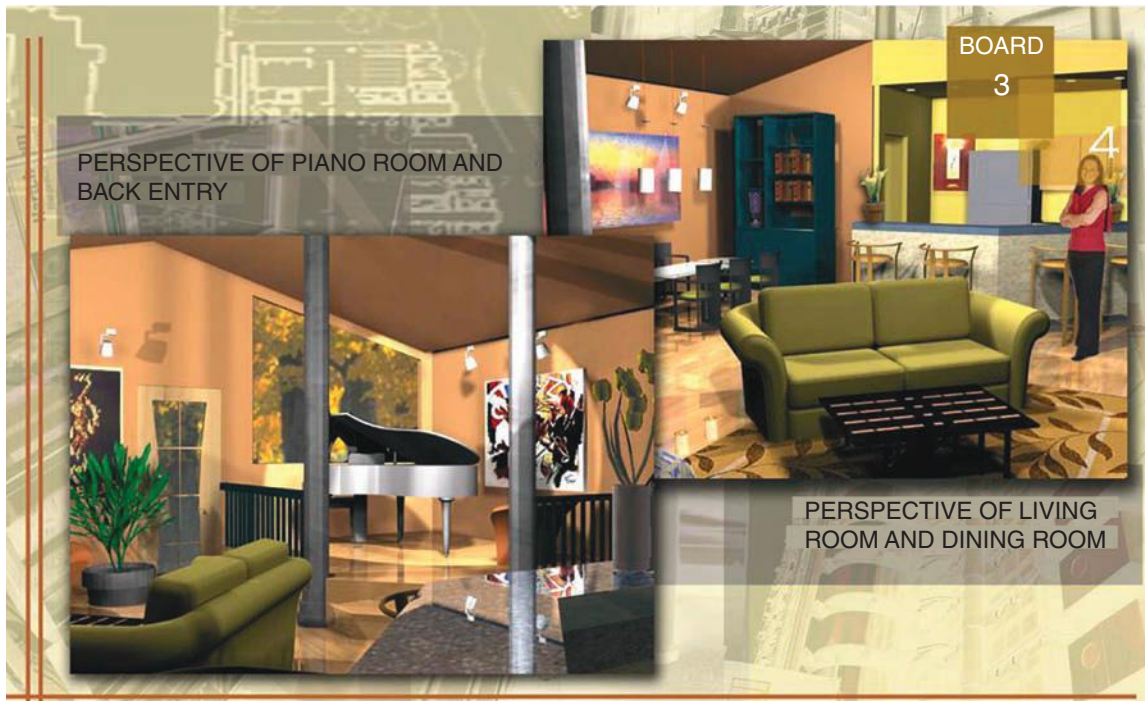
FIGURE 18.31 These computer renderings are presented in a two-point perspective, drawn with two vanishing points.
