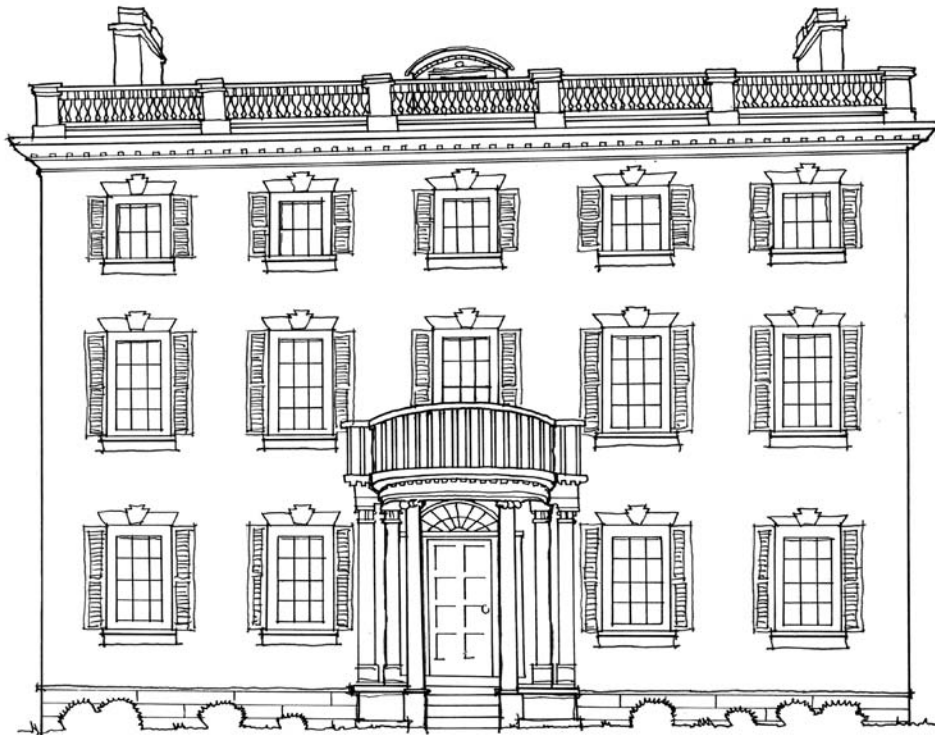
FIGURE 2.52 The Federal style produced a refinement of classical taste in American architecture. Symmetry, an entry portico, classical elements, and a roof topped by a balustrade are typical of this style.
