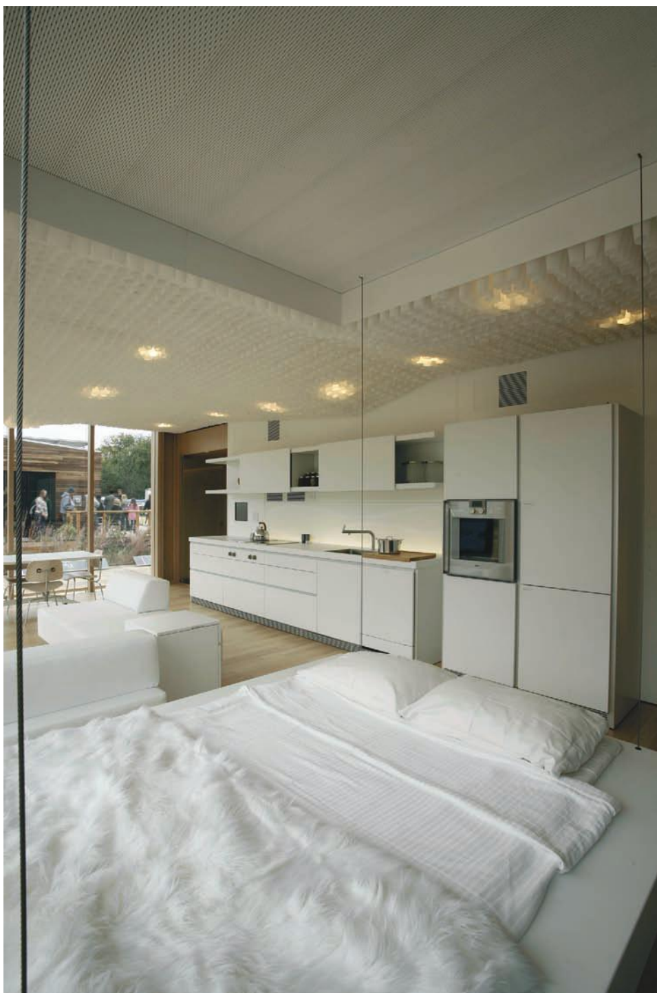
FIGURE 16.17 This bed lowers from its storage area near the ceiling by use of steel cables, to provide more living space when the bed is not in use.
