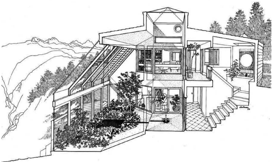
FIGURE 8.11 In passive solar design, interior spaces are often open to one another to encourage the natural flow of heat throughout the building.
